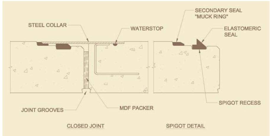
Figure 1. J Series Jacking Pipe Joint.
