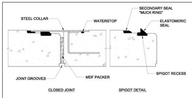
Figure 1 - J Series Jacking Pipe Joint
