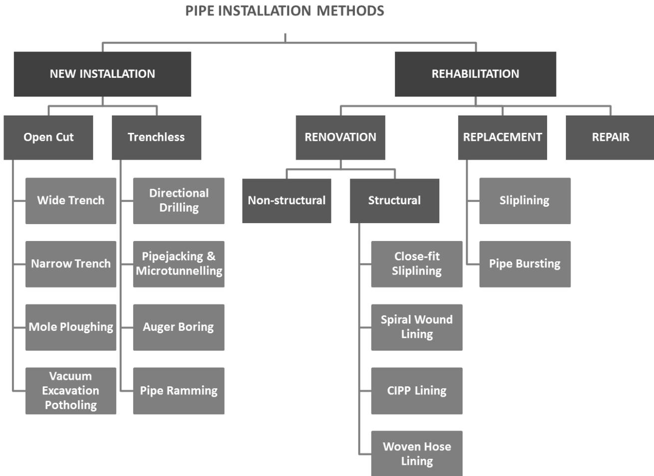
**Figure 1 - Pipe Installation Techniques (after ISTT Guidelines - <http://www.istt.com/guidelines>)**
