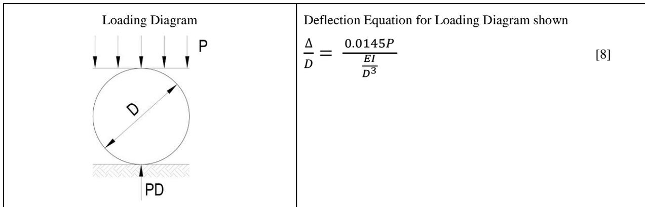
Figure 7 - Loading diagram and deflection equation for pipe with no side support (Watkins & Anderson)
