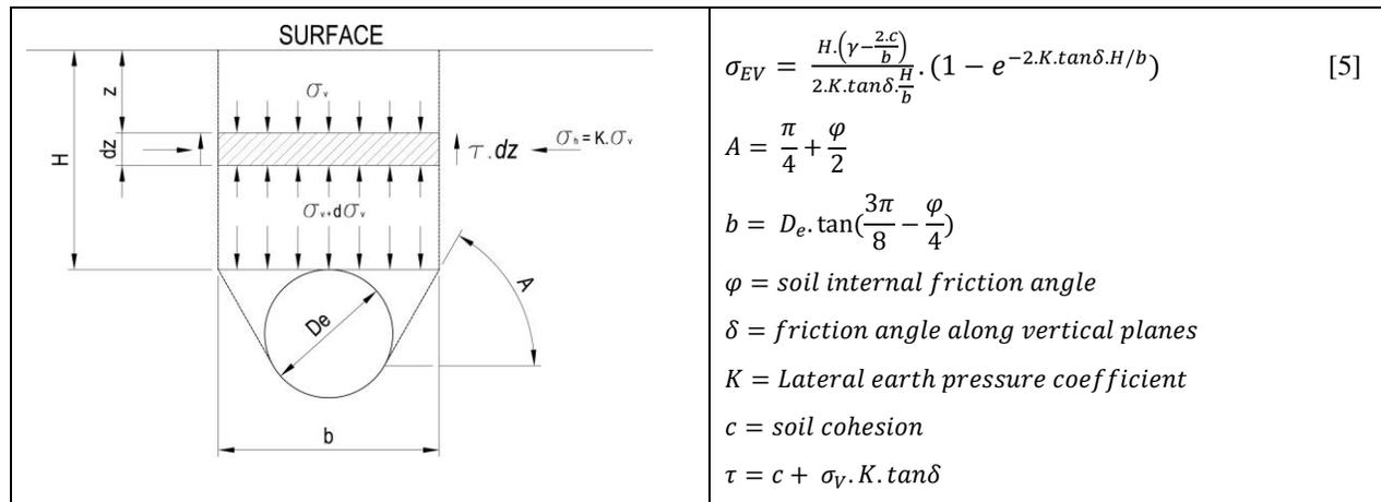
Figure 4 - General Terzaghi Model (after French Society for Trenchless Technology, 2006)
