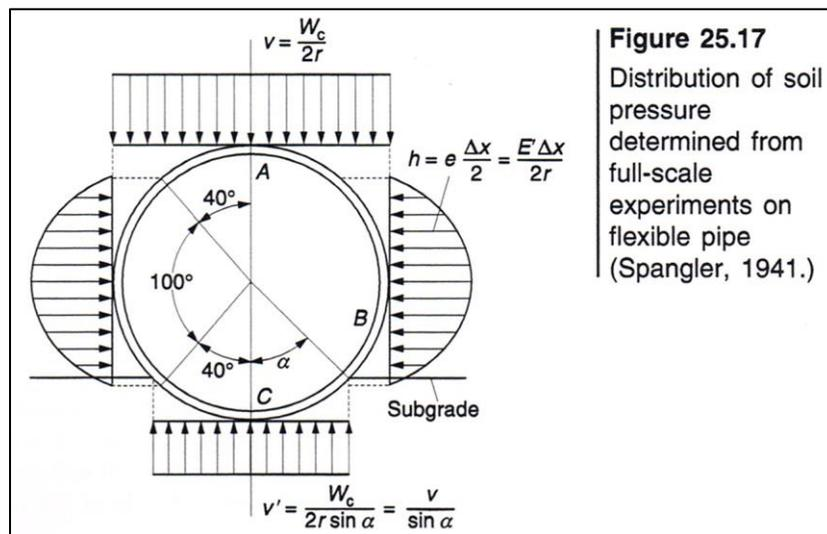
Figure 6 - Pressure distribution around pipe - modified Iowa Formula (Hardy & Spangler, 2007)
