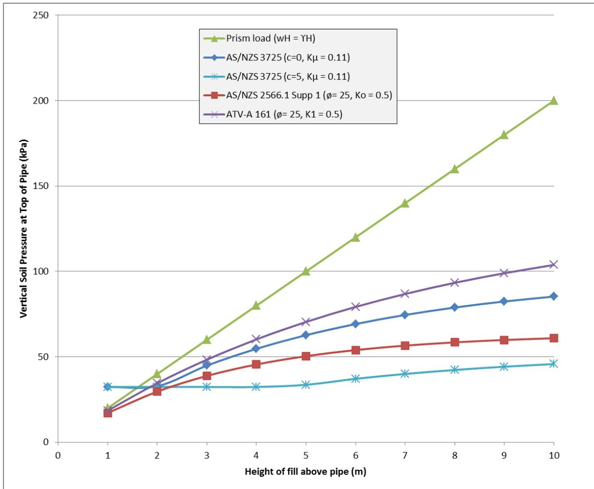
Figure 5 - Comparison of Vertical Soil Pressures Using Different Methods
