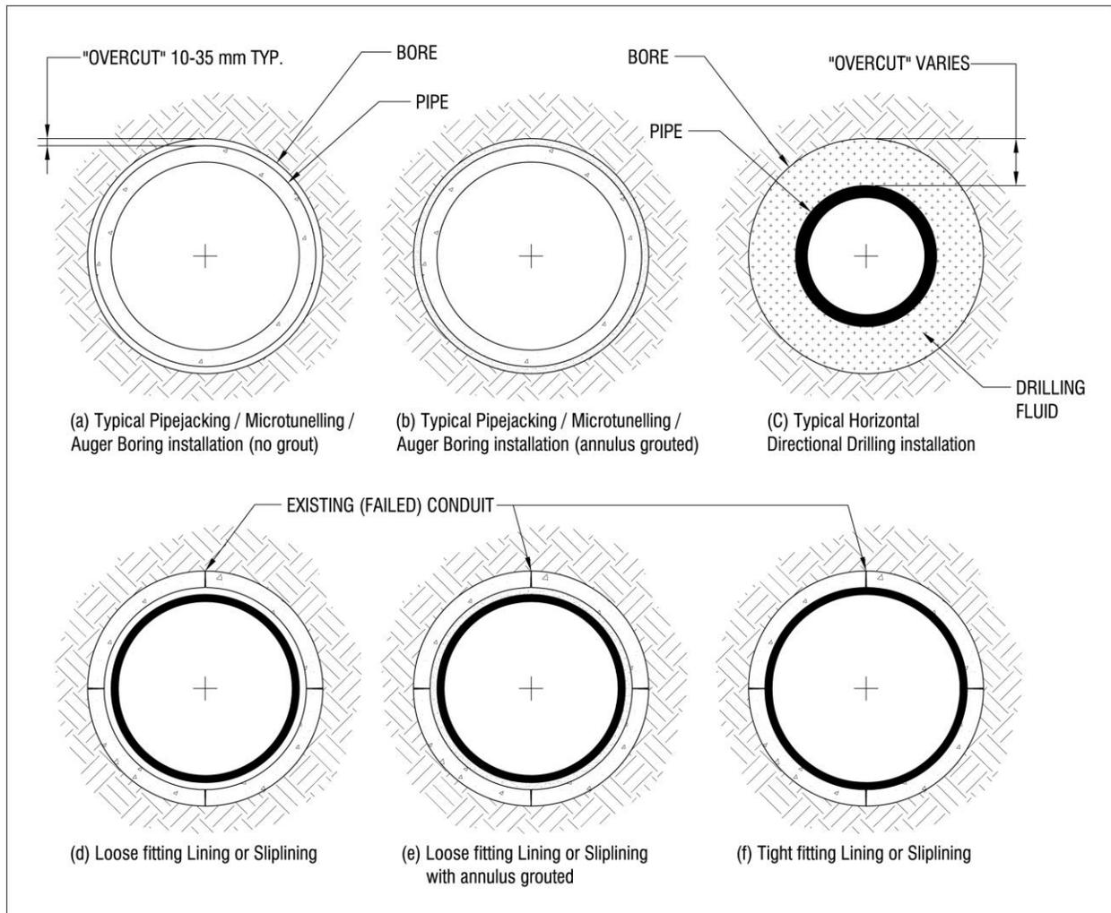
Figure 2 - Typical "pipe" installations using Trenchless techniques
