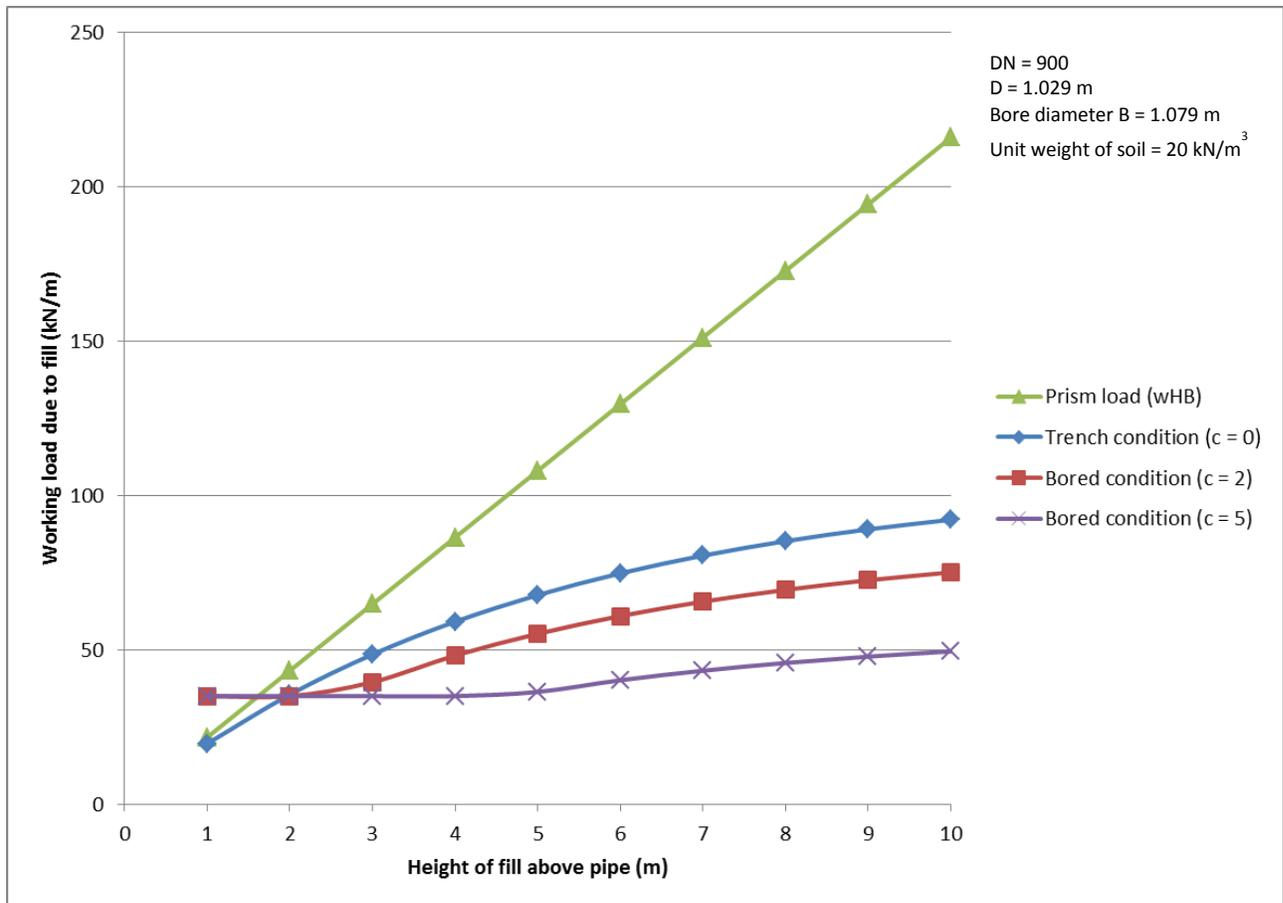
Figure 3 - Working loads due to fill for different installation methods
